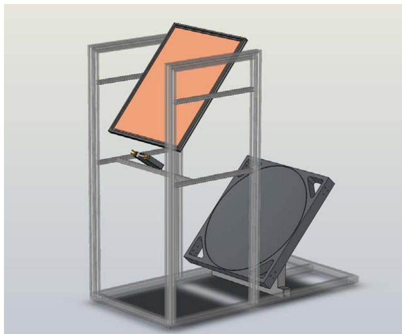
Fig 1. Model of new radio-wave imaging system.
