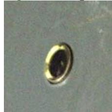
**Figure 2.** 1/8" B&K microphone in a baffle.
